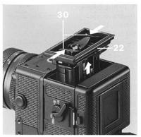
Press the two release buttons 30 together, pull out film insert 22 and remove the film cartridge.
