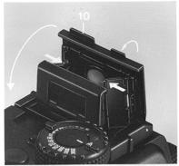
Closing the viewfinder hood: first fold the magnifier down by its grip, then fold in the two sidewalls and allow flap 10 to spring down.
