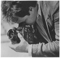
When using the viewfinder hood, the following method of holding the camera is recommended: one hand under the camera, the other free to operate the controls.
