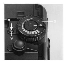
Switching on the automatic shutter speed control
