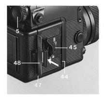
Pull out magazine drawslide 48 from masking slot 44 and slide into storage compartment 47. Set magazine switch 45 to SE and main switch 5 to »I«.
