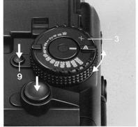
Set 1/2000s on control dial 3 after unlocking with button 9, so as to avoid slow shutter speeds occurring in poor light conditions. Press one of the shutter release buttons as many times as necessary to bring frame counter 18 to »1«. Then turn control dial 3 back to position »A«.
