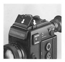
To replace the viewfinder hood, insert it tilted forwards, pushing against the spring pressure in the direction of the lens, and press down to engage.
